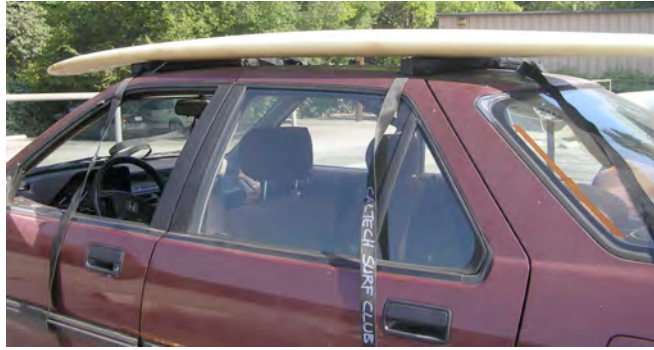
Figure 4: Place the surfboard with its fin facing up, and mass approximately centered over the two pads (perhaps slightly more towards the back of the car).
