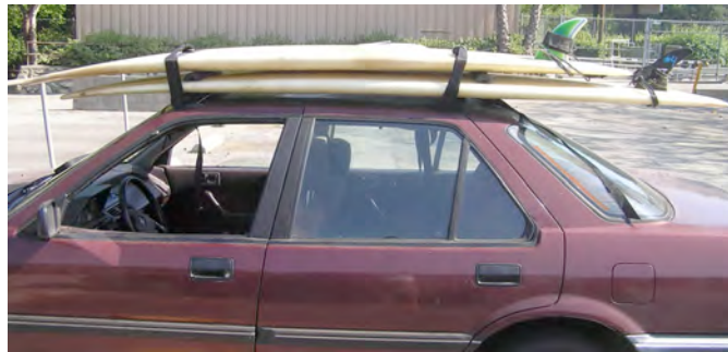
Figure 6: A pair of boards centered over the rack's two parts is most stable.
