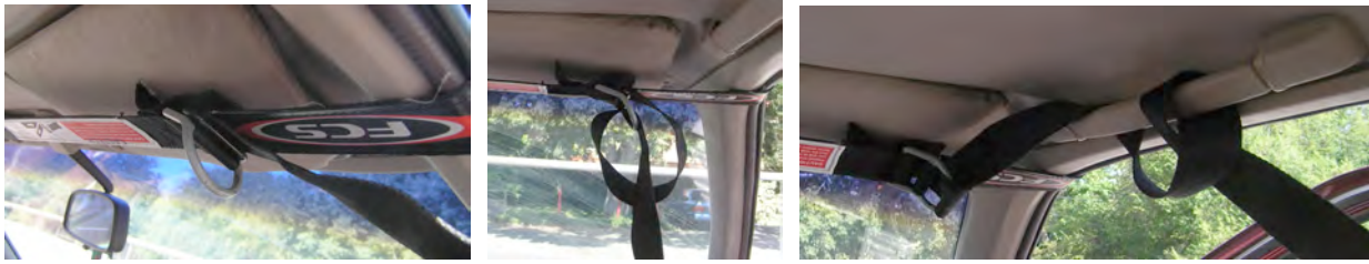
Figure 2: Attach the long strap to the buckle inside the car (see Figure 7 how to use the buckle), and always use a safety after tightening the strap tightly. Tuck away the excess strap.
