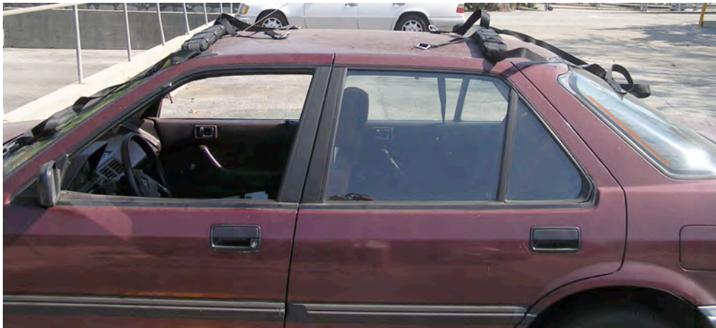
Figure 3: The two pieces of the rack securely and tightly attached to the car, so as to be as far apart as possible.
