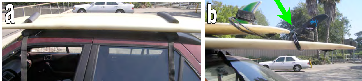
Figure 5: Foam padding between the boards is essential ( 5a ). Put one pad above each part of the rack, so it will be underneath where the strap runs. Make sure the fin of one board never touches the back of the board on top ( 5b ).
