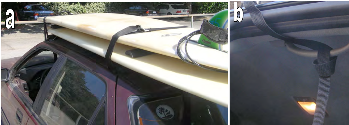
Figure 8: (a) Straps tightened, with safety knots, and the excess strap tucked into the car. (b) You can wrap the excess around the handle to keep it out of the way.
