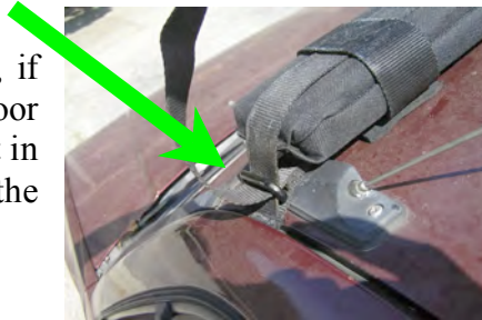
Figure 2: Attach the long strap to the buckle inside the car (see Figure 7 how to use the buckle), and always use a safety after tightening the strap tightly. Tuck away the excess strap.
