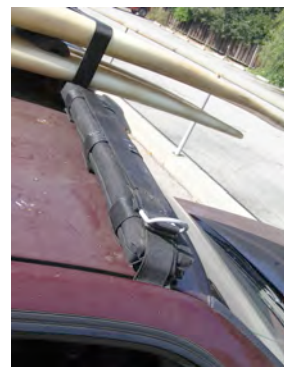
Figure 8: (a) Straps tightened, with safety knots, and the excess strap tucked into the car. (b) You can wrap the excess around the handle to keep it out of the way.
